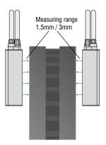
CSH1,4FL/4CH sensors enable robust and high precision multi-track measurements with very little installation effort.
