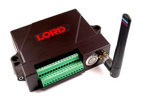
The V-Link-200 is a versatile wireless sensor with 4 differential and 4 single-ended analog input channels. It includes onboard PGA's, filtering, and a high-resolution ADC for precise measurement of a large range of sensor types, including strain gages, load cells, pressure transducers, and accelerometers.
