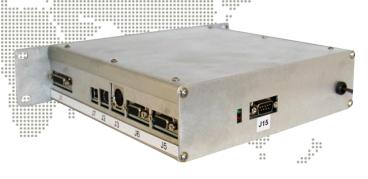
connected to the electronic control unit are automatically recognized by the system, their limits are automatically detected and their automatic calibrations can be performed. Besides this feature, the system also allows manual calibration of third party sensors. The sensor measurement resolution of the electronic control unit is 24 Bit.
