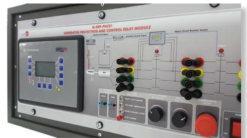
Automatic voltage and speed controller (AVR, ASC) detail
