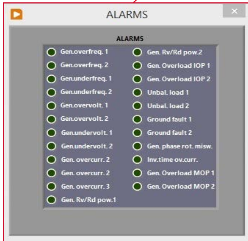
Generator alarm panel.
