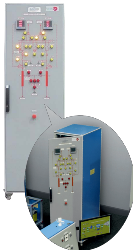
LTS2. Line III and IV Cabinet with Transmission Substation with Protection Relays System
