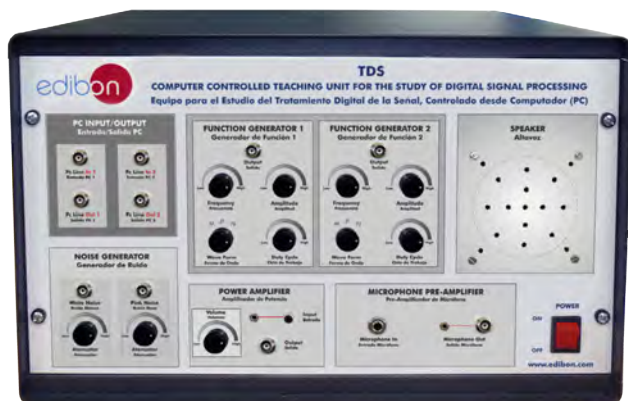
① Unit: TDS. Computer Controlled Teaching Unit for the Study of Digital Signal Processing
