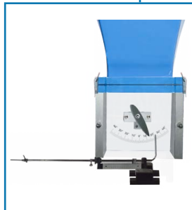
ATB/D.F. Model to Study the Drag Forces
