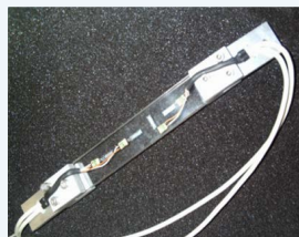
N°10-G. Small Rectangular Specimen with strain gauges + N°10. Small Rectangular Specimen
