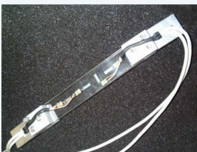
N°9-G. Medium Rectangular Specimen with strain gauges + N°9. Medium Rectangular Specimen
