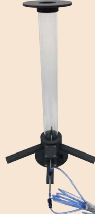
HVCC-CTPP. 64 mm diameter duct and pressure taking with Pitot
