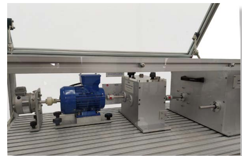
Assembly of the Set to Study Damage in Gears "MDU-SSDG" in the Computer Controlled Machine Diagnosis Unit "MDUC" with Break and Load Unit "MDU-BLU"
