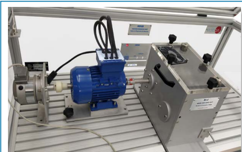
Assembly of Set of Electromechanical Vibrations, "MDU-SEV", in the MDU Base Unit, "MDU-UB", with the Break and Load Unit, "MDU-BLU".
