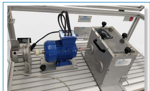
Assembly of Set of Electromechanical Vibrations, "MDU-SEV", in the MDU Base Unit, "MDU-UB", with the Break and Load Unit, "MDU-BLU".
