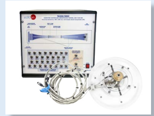
TA300/300C-TARC. Force Measurement Interface and Sensors, range: 0 – 2.5 kg (requires at least one resistance model or an airplane model)
