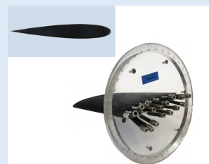
TA19/300. Pressure Distribution in a Wing Model with NACA 0015 Profile
