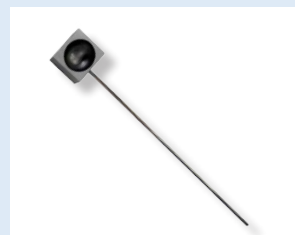
TA9/300. Drag Model of Hemisphere Concave to Airflow (requires the model TA300/300-TAR)
