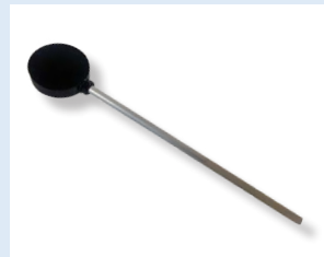
TA3/300. Circular Plate Drag Model (requires the model TA300/300-TAR)
