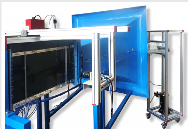
APIV/30. PIV 2D flow Visualisation for Velocities up to 30 m/s and Area of 100 x 100 mm
