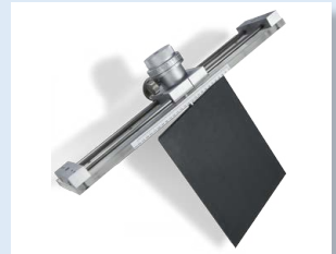
TA300/300-BLE. Model to Study the Boundary Layer in a Flat Plate (requires the model TA17/300)
