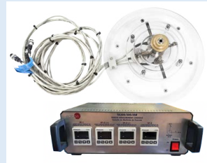
TA300/300-TAR. Force Measurement Console and Sensors, range: 0- 2.5 kg (requires at least one resistance model or an airplane model).
