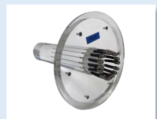
TA22/300. Pressure Distribution in a Cylinder
