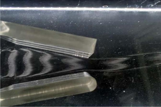
Velocity increase when the passage section of the flow.
